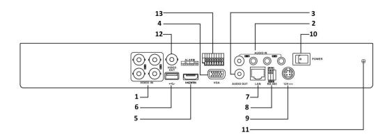
The rear panels of DS-7208HUHI-F2/N and DS-7216HUHI-F2/N provide 8 and 16 video input interfaces respectively.
