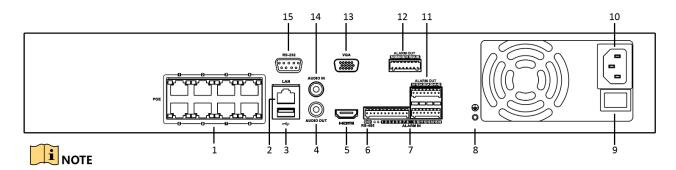
The DS-7716NI-Q4/16P and DS-7732NI-Q4/16P provides 16 network Interfaces with PoE function.
